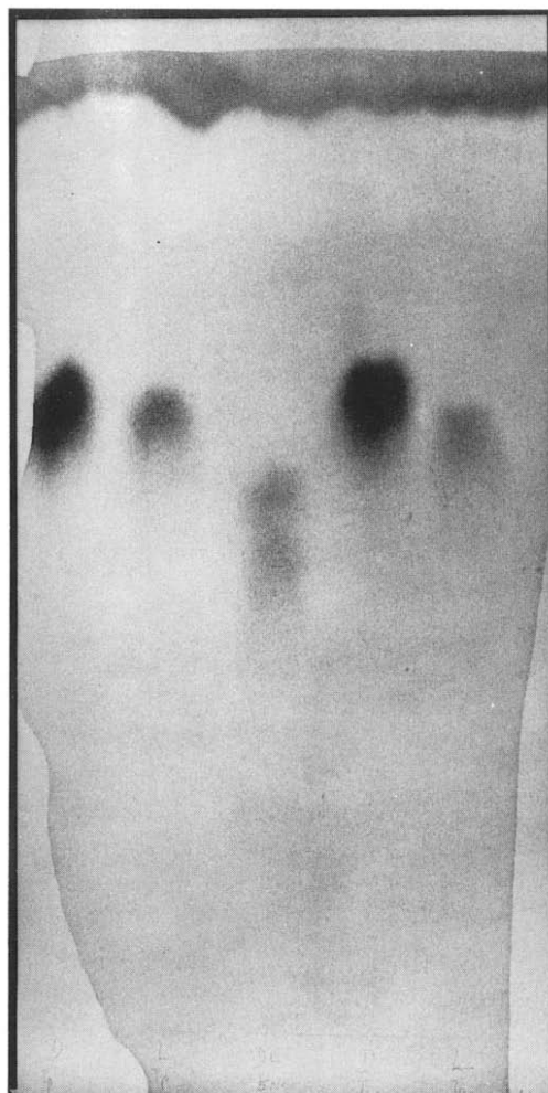
Fig. 4. Chromatogram of (from left to right) D-tryptophan, L-tryptophan, DL-5-methyltryptophan, D-tryptophan and L-tryptophan on Whatman 3MM paper, 40-cm long, with 1 M NaCl.
